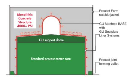
Simple, labour saving set-up of GU Manhole Base Liner with Sealplate for producing fully lined, monolithic manhole bases.
